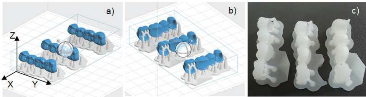
Fig. 2. Manufacturing of dental bridges by 3D printer “Form 1+”: design of 3D virtual models – a) and b) and as-printed bridges – c)
