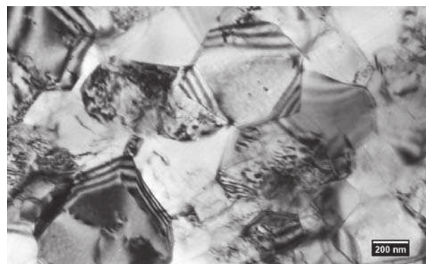
Fig. 8. Titanium substructures after three passes through Conform equipment ( n = number of passes)
