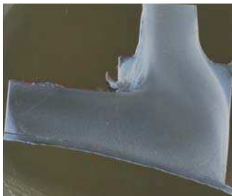
Fig. 3. Metallographic investigation – macro of the Ti feedstock section in the chamber die
